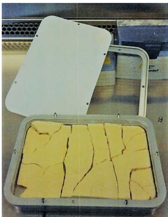
Fig.: Lyophilization cake in the Lyoprotect® Tray
